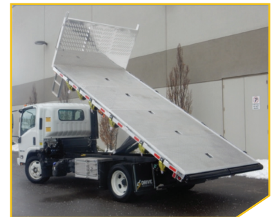
Chassis: Isuzu NRR (Shown: 16' Aluminum Dumping Deck)
